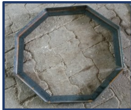
Fig. A.2 Base octagonal soldada.
